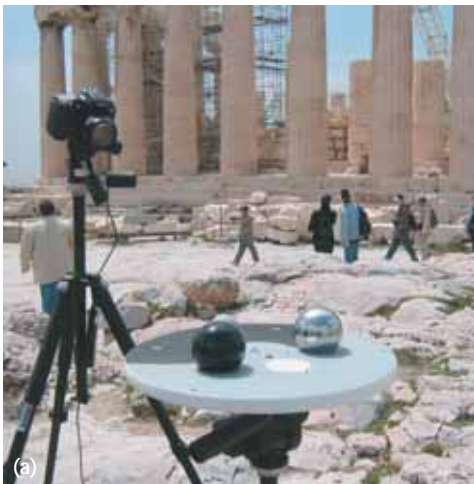
Figure 7. Capturing the lighting and geometry of the Parthenon. (a) A light probe device records incident lighting conditions near the base of the temple. (b) A 3D surface model of the scene geometry obtained using 3D laser scanning.
